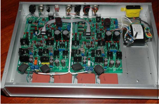
37. Output capacitors: 0.01u K40Y-9//Silmic BP – custom made//10u PIO MBGO.
