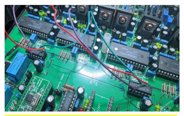
Added by Spencer: Indeed there is no need to solder the wires to the U4 and U11. In the output of the digital filter, can make use of the 4 output pins (23 to 26) and then connect to the output of USB board. See circuit below: Of course you have to remove the digital filter chips first!
